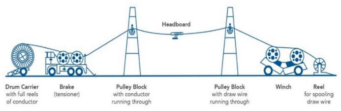
Note: Schematic illustration only. The location of the brake and winch components could be several kilometres apart.
