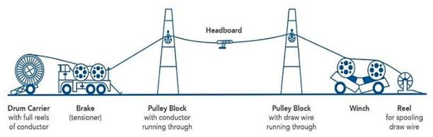
Note: Schematic illustration only. The location of the brake and winch components could be several kilometres apart.
